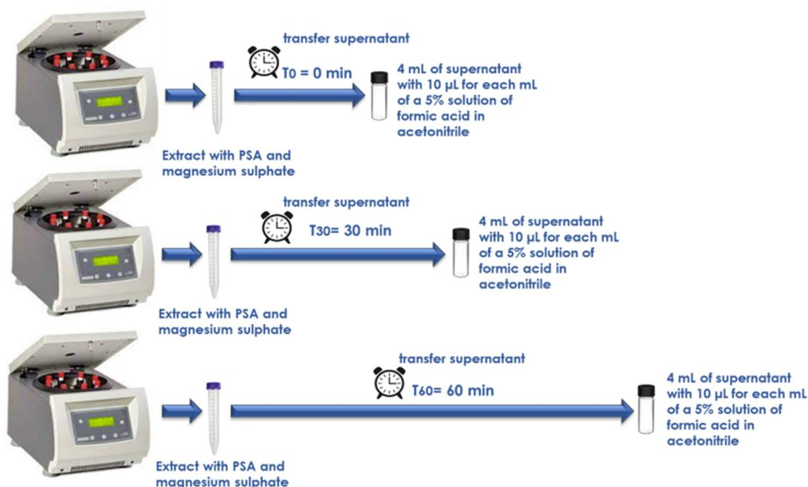
**Figure 1.** Scheme of experiment A
